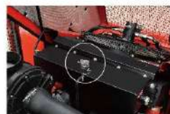
• Easy cooling liquid adding and check
